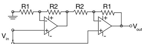
Diagram 8. High common mode voltage rejection unity gain differential amplifier
