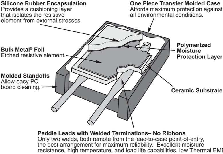
The combination of ruggedized leads and molded case, plus the highly efficient heat transfer characteristics of the unique assembly and the ceramic substrate results in a high reliability resistor with excellent moisture resistance, high temperature, and load life capabilities. These also afford a very low Thermal EMF.
