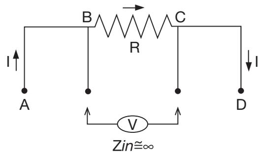
The four-terminal device separates the current leads from the voltage-sensing leads. This configuration eliminates the effect of the lead wire resistance from points  $A$  to  $B$  and  $C$  to  $D$ . Overall, Bulk Metal® Foil technology provides performance capabilities far greater than any other resistor technology can supply in a product of comparable size.
