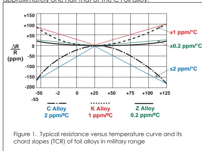
Figure 1. Typical resistance versus temperature curve and its chord slopes (TCR) of foil alloys in military range
