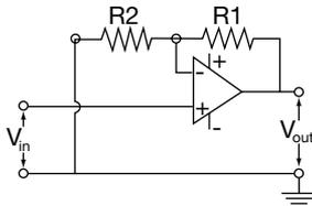
Diagram 4. Instrumentation AMP w/ Shield Driver
