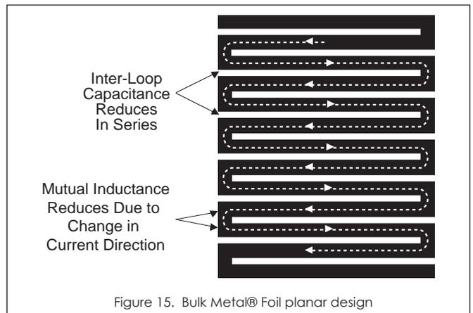
capacitance produce reactance proportional to the operating frequency, which changes the effective resistance and the phase between the current and voltage in the circuit.
