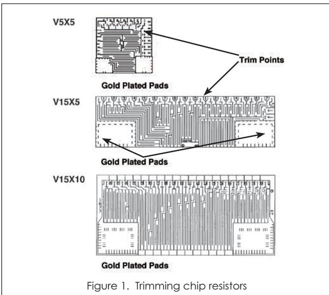
Figure 1. Trimming chip resistors
