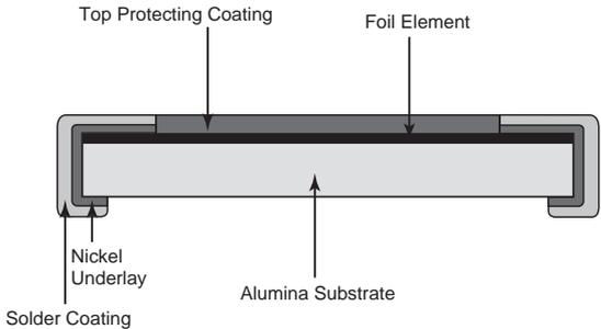
Figure 24. Surface-mount wrap-around chip foil resistor construction
