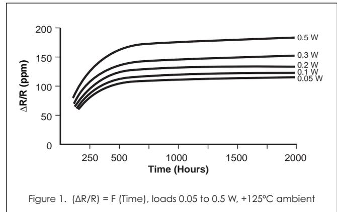
Figure 1.  $(\Delta R/R) = F(\text{Time})$ , loads 0.05 to 0.5 W, +125°C ambient
