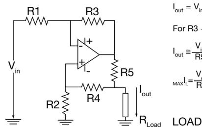
Diagram 7. Differential input instrumentation amplifier
