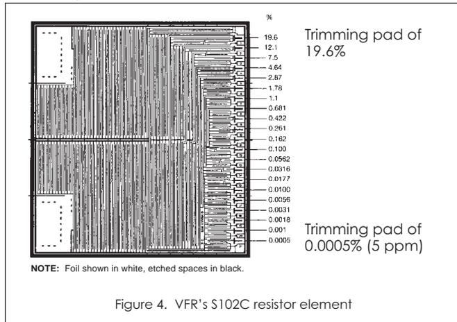
Figure 4. VFR's S102C resistor element
