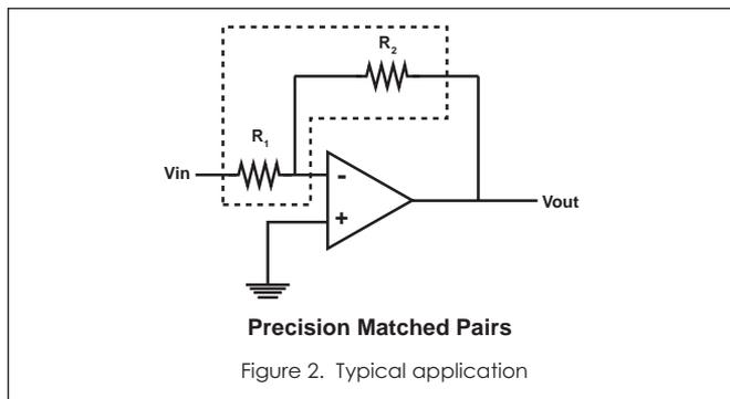
The best analog design would be to use a fundamentally low-absolute-TCR resistor, since it would minimize the effect of ambient temperature and self-heating. This is impossible to accomplish with resistors with high TCR  $>5$  ppm/°C, even with good initial TCR tracking of less than 2 ppm/°C.
