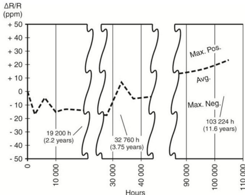
Figure 3: S102C (Bulk Metal® Foil Resistor) 1kΩ over 10 years, actual tests.
