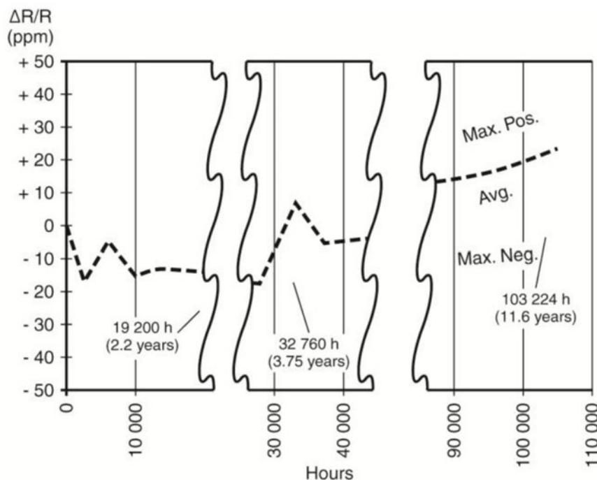
Figure 3: S102C (Bulk Metal® Foil Resistor) 1kΩ over 10 years, actual tests.
