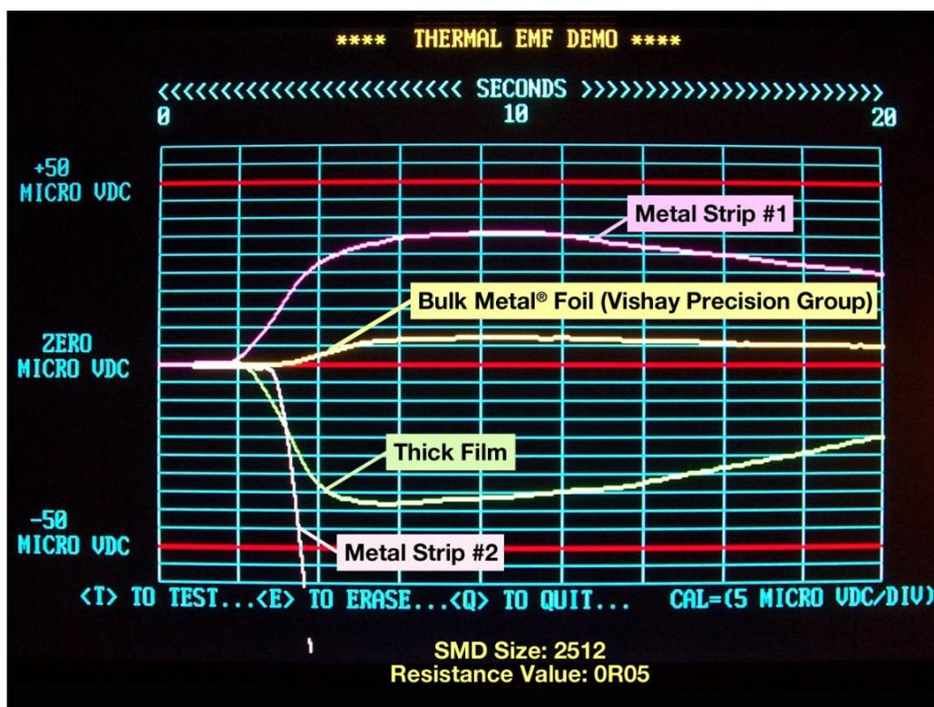
Note: S102C/K and Z201, Z203 resistors have a thermal EMF of only 0.1 $\mu$ V/°C
